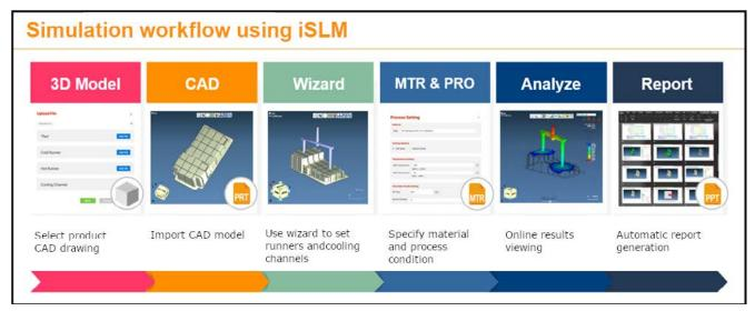
iSLM offers various mold flow analysis automation features, significantly simplifying the operation process for rapid design verification and optimization.
