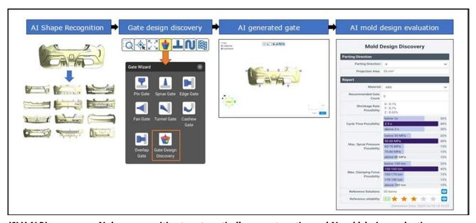
iSLM AI Discovery uses AI shape recognition to automatically generate gating and AI mold design evaluation.
