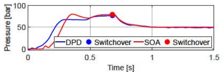
Figure 9: Hydraulic load pressure as a function of time for the case of late switchover.
