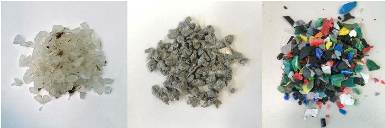
Figure 1: The tests were carried out on three different materials: pellets of virgin PP (left), PP agglomerate obtained from post-consumer film (center) and regrind obtained from HDPE beverage closures (right).
