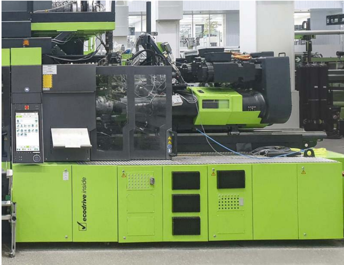
Test setup at the pilot plant in St. Valentin: for the two-stage process, ENGEL has combined a plasticizing screw with an injection screw.
