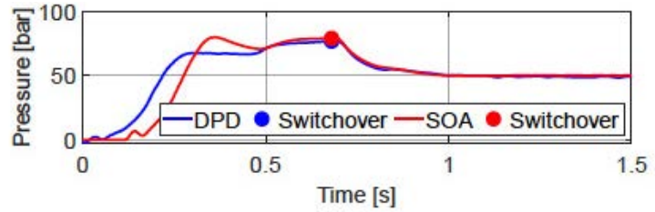
Figure 7: Hydraulic load pressure as a function of time for the case of early switchover.
