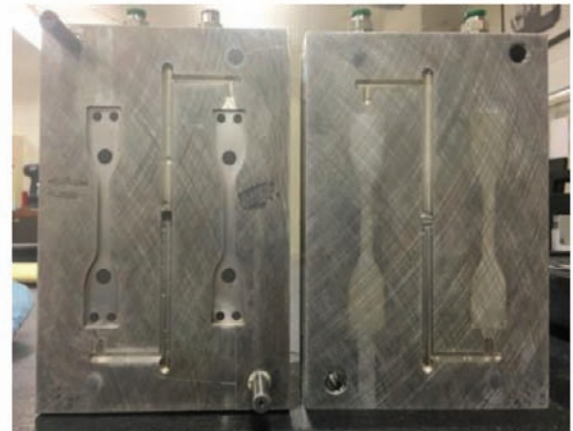
Figure 1: Fabricated Mold According to ASTM.
