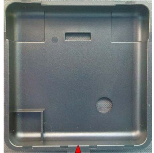
Figure 1: A specimen part with ribs, wall thickness variations and holes was used for the analysis of weld lines and surface roughness (view: rear side). The red triangle marks the gate. Photos courtesy of ENGEL.
