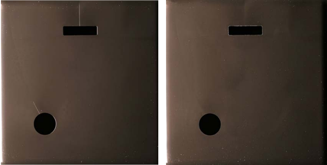
Figure 3: The variothermal processing prevents visible weld lines. The PC+ABS part was manufactured with a cavity insert temperature of 90 °C (left, without variothermal control) and 170 °C (right, with variothermal control).
