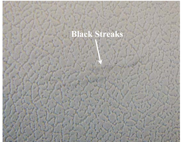
Figure 7: Photograph of the black colored streaks in a PP molded part.
