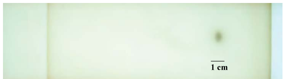
Figure 5: Photograph of a cabinet section without the masterbatch colorant, showing degraded resin that was responsible for color streaks.
