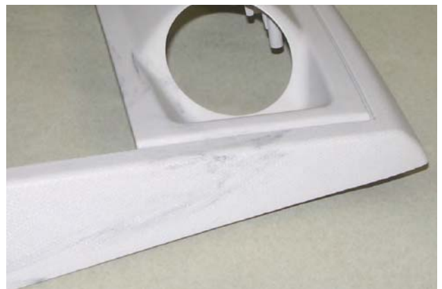
Figure 1. Photograph of a beige colored automotive interior part that was scrapped due to black speck contamination.
