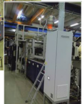
SyncroSpeed 135 HP 2-motor system installed on a Cincinnati 723t.
