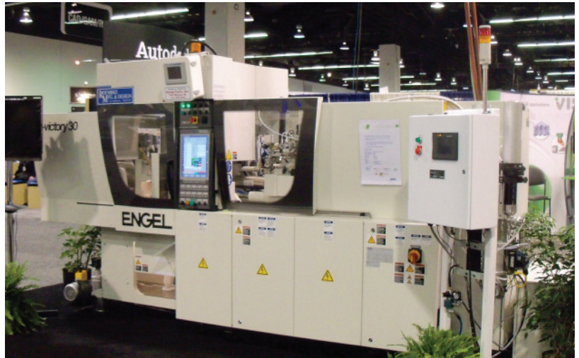
Figure 2: An Engel e-victory 80/30 hybrid tiebarless machine was used for this study. X-melt is a software add-on that requires no hardware modifications. The software can be turned off when not needed.
