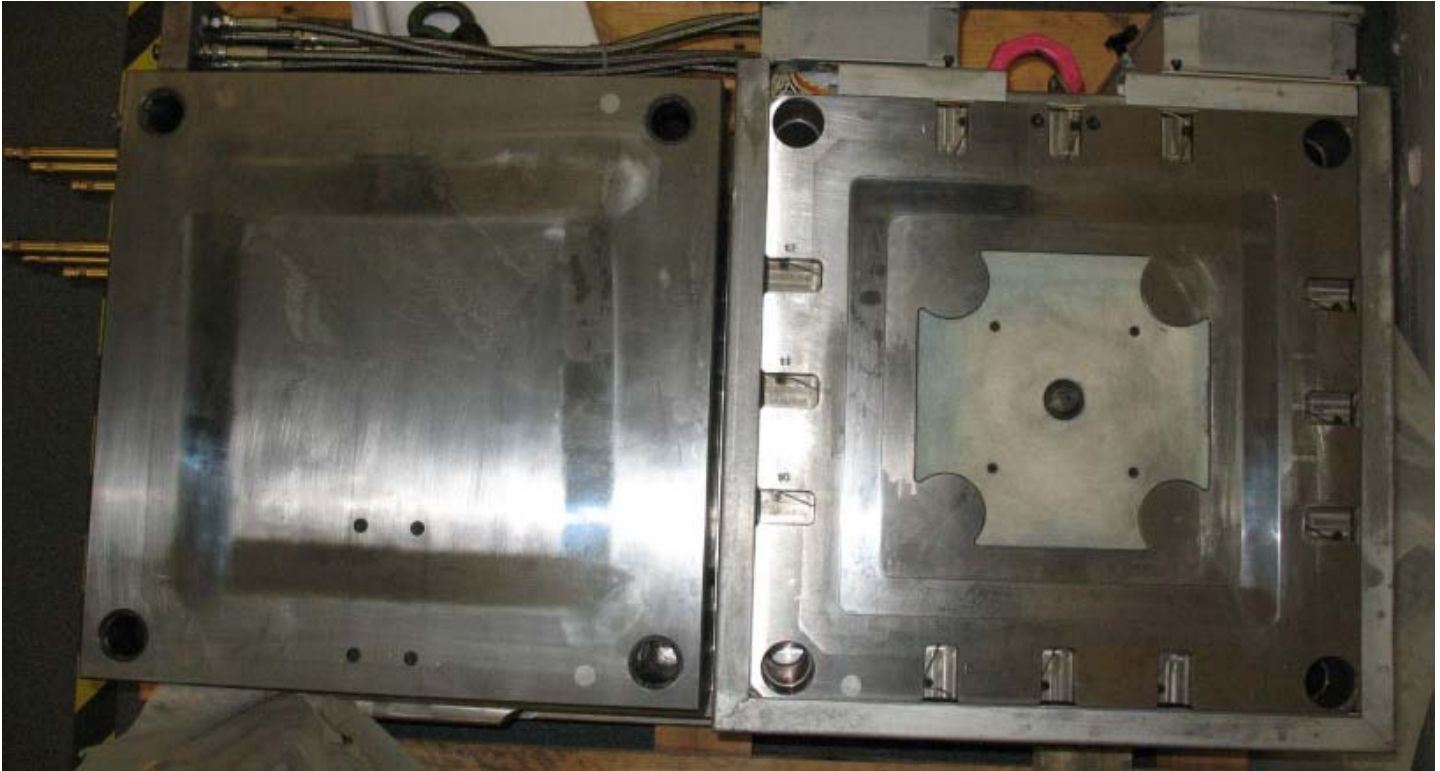
Figure 4 (above): The new RHCM mold with rotary plate.
