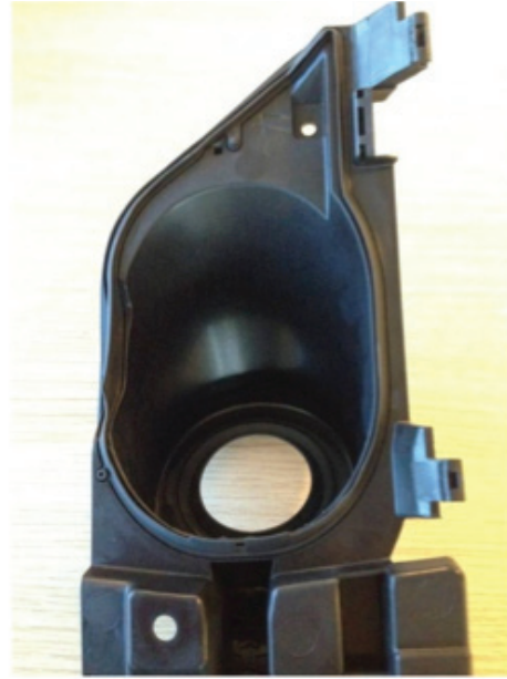
Figure 7: Both simulation (left) and experiment (right) result in short-short-free filling in the final design.
