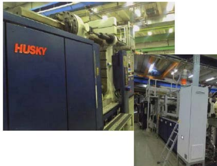
SyncroSpeed 250 HP single-motor system installed on a Husky 1100t
