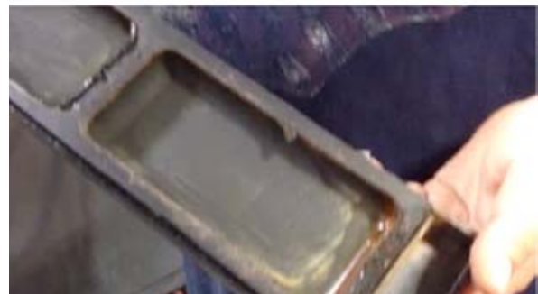
Image 2: DTEA II™ tested chiller surfaces free from slime
