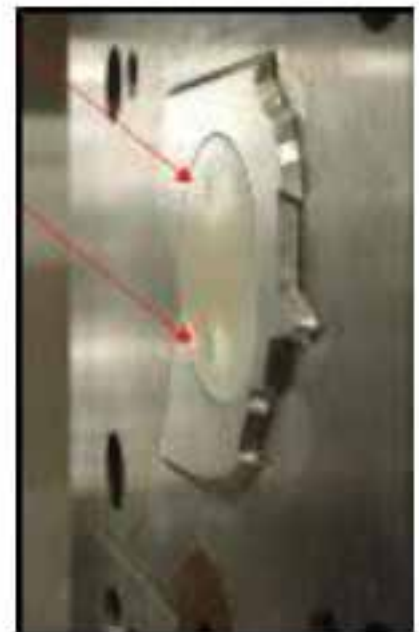
Figure 7: Tool deformation on different wall thicknesses
