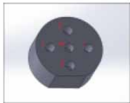
Figure 5: Hole Depth Insert (Back side is pictured) in Solidworks. Labeled with the corresponding tool thicknesses:
