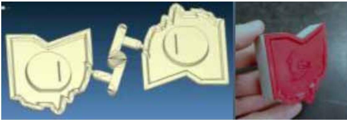
Figure 1: Moldex drawing of the lid and final molded lid/box assembly
