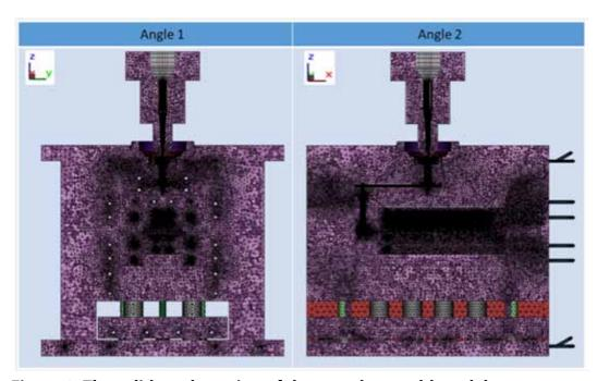
Figure 3: The solid mesh section of the complete mold model.
