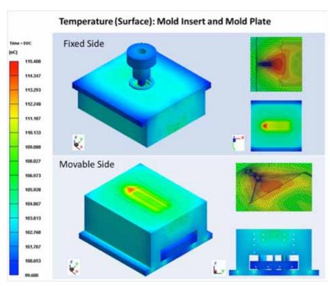
Figure 5: The temperature distribution of the mold inserts and mold plates.
