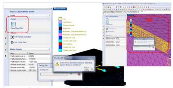
Figure 4: Mesh cell intersection check before mesh export.
