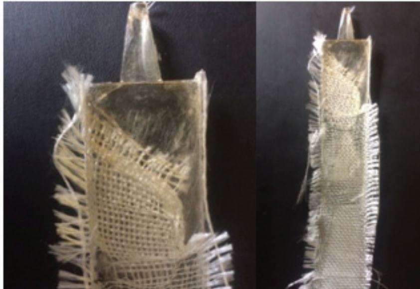
Figure 4: Degradation of polycarbonate and misalignment cause for flow advanced.
